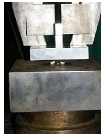
Figure 7. Test-piece tested on Zwick-Roell Z005 universal testing machine.
